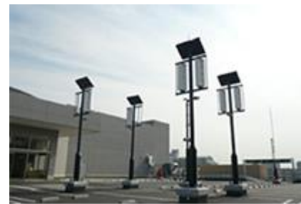
Savonius wind turbines with solar panels
