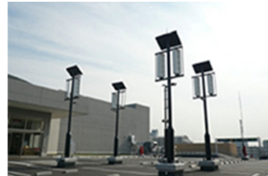
Savonius wind turbines with solar panels
